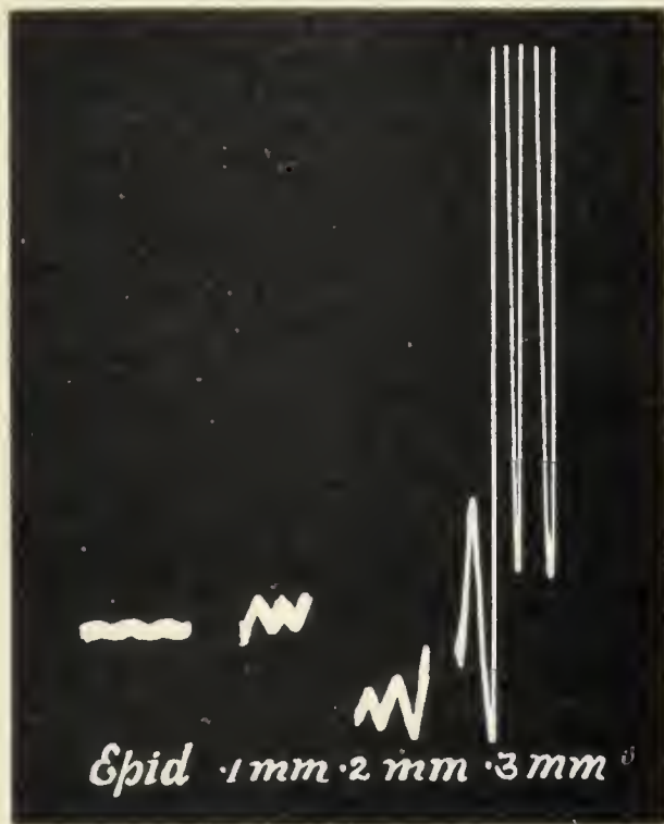
FIG. 211. Record showing the amplitude of electric pulsation in different layers of stem of Impatiens .
